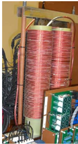
Figure 2. 750 kW 50 kHz transformer based on a nanocrystalline core with litz-wire windings, in a test bay at Princeton Power’s facility.
